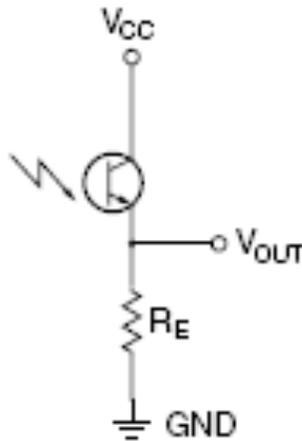
**Figure 2. Common-Collector Amplifier**
