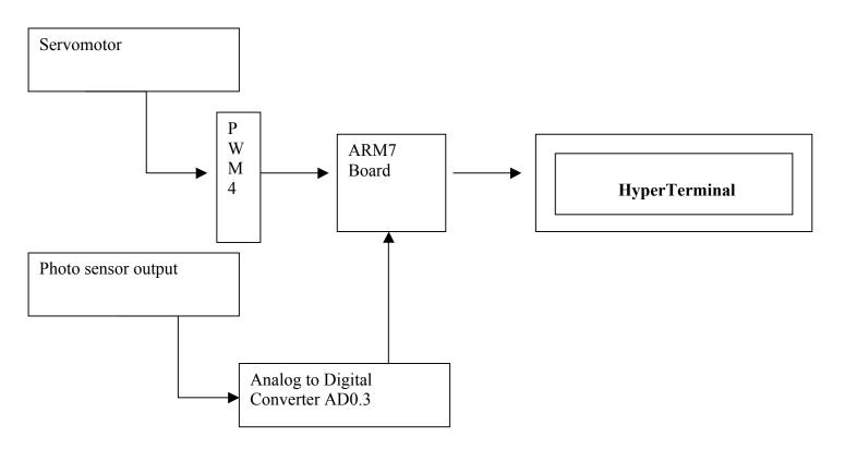
Figure 1: Connection Diagram
