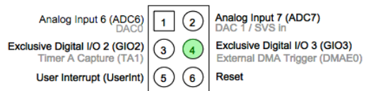
Figure 21 : Functionality of the 6-pin expansion connector (U28).
